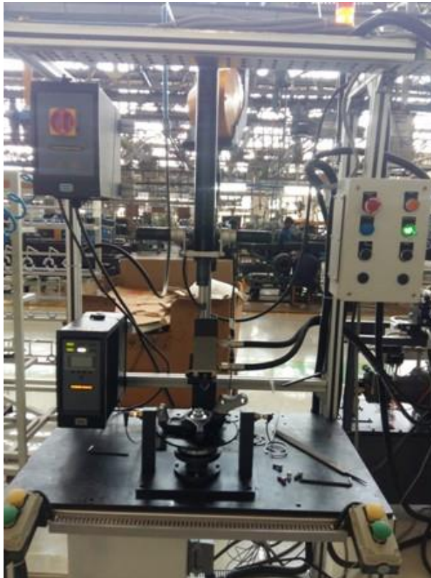
Automated inline DC torque wrench automation
